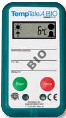
The TempTale<sup>®</sup>4 BIO (TT4 BIO) is a compact, battery powered ambient electronic temperature monitor designed with a higher degree of accuracy to meet critical pharmaceutical applications for monitoring temperature-sensitive products during storage and transportation. The TT4 BIO helps to assure the quality, safety and efficacy of temperature-sensitive products in storage and transit by
